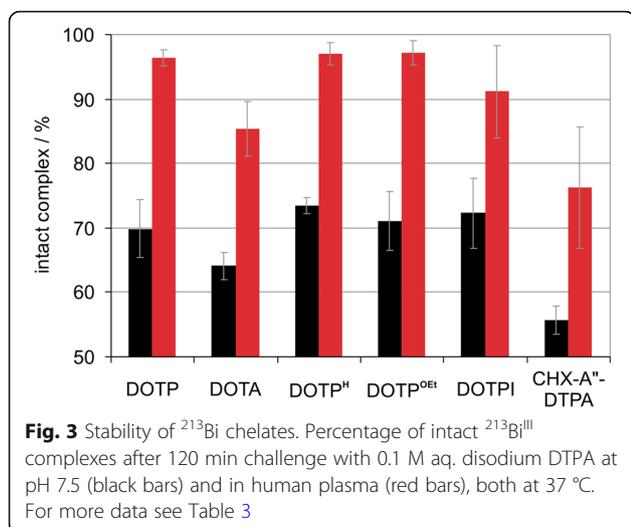
competing medium at 37 °C. The fraction of intact chelate was evaluated by radio-TLC. Values were normalized to the fraction of radiometal complex at  $t = 0$ .
