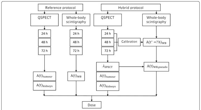
**Fig. 2** Illustration of the reference protocol (RP) and the proposed hybrid protocol (HP); for the hybrid protocol, the sequential whole-body planar imaging is replaced by a single whole-body planar acquisition at an appropriate time point at 24, 48, or 72 h p. i. (HP24, HP48, HP72); QSPECT indicates quantitative SPECT
