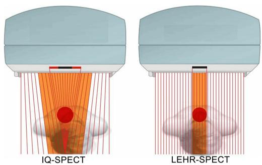
Fig. 1 Schematic diagrams of IQ single-photon emission computed tomography (SPECT) and low-energy high-resolution (LEHR)-SPECT
